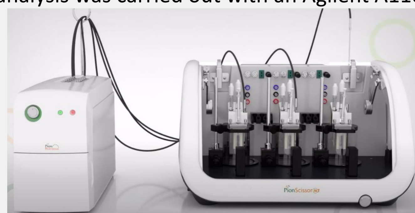
Figure 1. The Pion SCISSOR® (right) and Rainbow® R6 (left) systems were used to monitor in situ release of a formulation.
