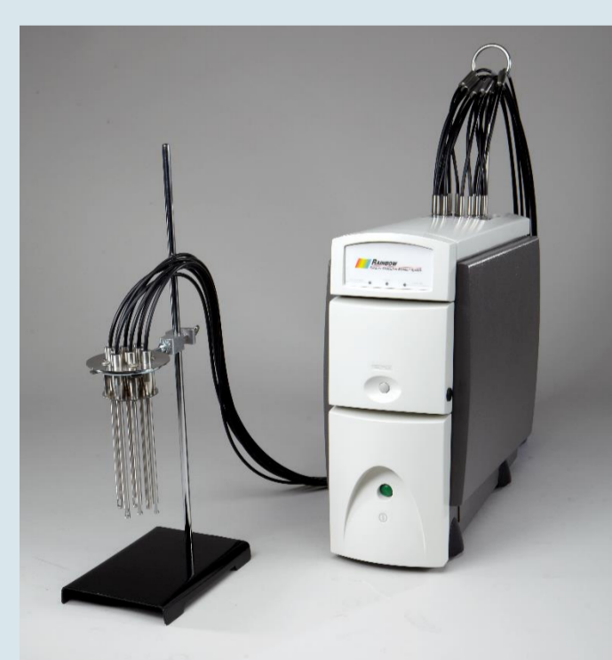
Figure 1. Rainbow ® instrument (Pion Inc.) shown with standardization station collects 8 full UV-Vis spectra (200 – 720 nm) in less than 2 seconds.
